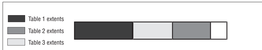
Figure 6-13. A Dbspace Reorganized to Eliminate Interleaved Extents
